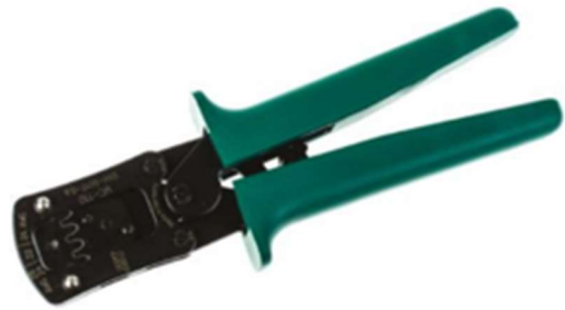
9) Optional: Connector Plug, Pins and crimper (Usually JST XHP-2, varies based on aircon model)
